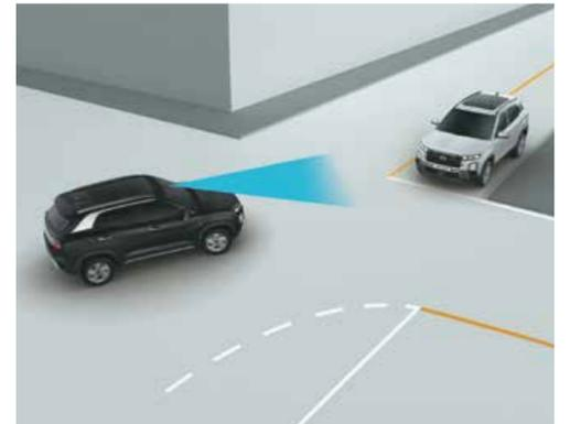
Forward Collision - Avoidance Assist - Junction Turning (FCA-JT)
