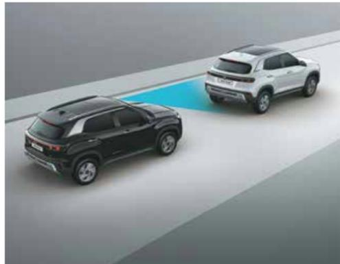
Forward Collision - Avoidance Assist - Car (FCA-Car) & Forward Collision Warning (FCW)
