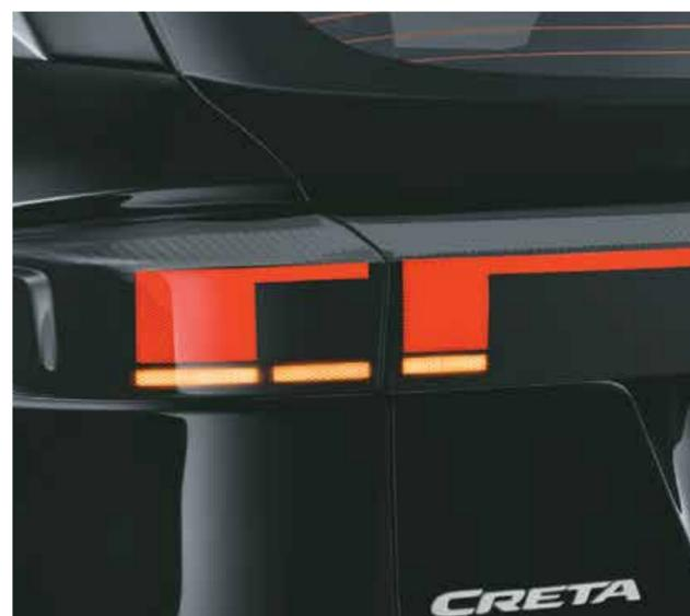
LED rear turn signal with sequential function
