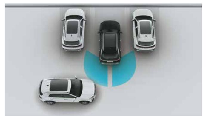
Rear Cross - Traffic Collision - Avoidance Assist (RCCA) & Rear Cross - Traffic Collision Warning (RCCW)
