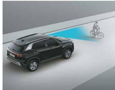
Forward Collision - Avoidance Assist - Cycle (FCA-Cyl)
