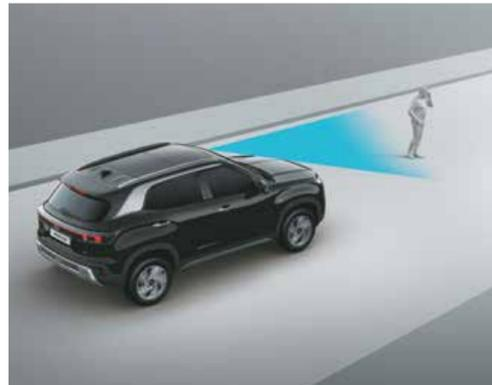
Forward Collision - Avoidance Assist - Pedestrian (FCA-Ped)
